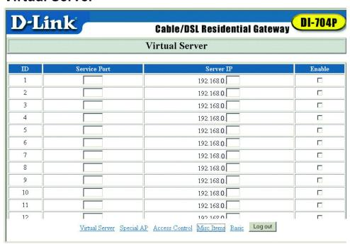
The firewall filters out unrecognized packets to protect your Intranet; so all computers networked with the DI-704P are invisible to the outside world. If you wish, you can make some of them accessible by enabling the *Virtual Server Mapping*.
